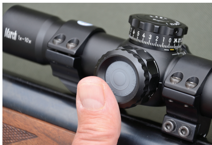
Pressing the centre of the parallax drum illuminates the reticle
