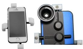
First loosen the lock knobs on each support arm. Between the support arms, align your smartphone's camera lens to the adapter's body hole. Adjust each support arm position to secure your phone as shown. Once an arm is in the desired position, tighten its lock knob. Once all 4 arms have been adjusted, verify that your smartphone is secured to the adapter body and that it will not fall out.
