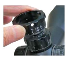
Lock the 3 screws of the large dial using Allen wrench.
