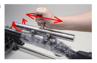
(7) The lapping bar gets dirty like this. After the work is completed, wipe off the compound cleanly.
