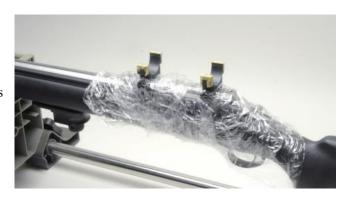
(5) Apply lapping compound to the inside of the mounting area at the bottom of the ring.
