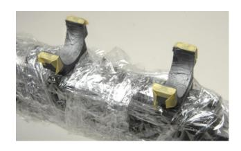
(6) Move the lapping bar moves back and forth and rotate it to align the front and rear rings.
