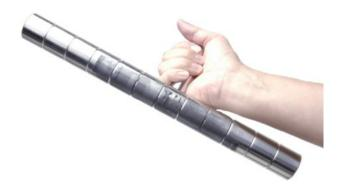
(8) The inside of the lower part of the ring will look like this after wiping off the compound. It is not necessary to make it smooth and shiny. The right amount of roughness must remain. Make sure to cleanly wipe off the compound. After this, apply a small amount of compound to the inside of the upper half of the ring and lightly wrap the ring in your hand.
