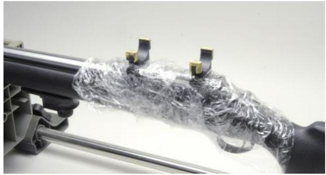
(5) Apply lapping compound to the inside of the mounting area at the bottom of the ring.
