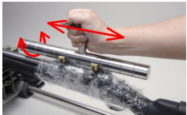
(7) The lapping bar gets dirty like this. After the work is completed, wipe off the compound cleanly.
