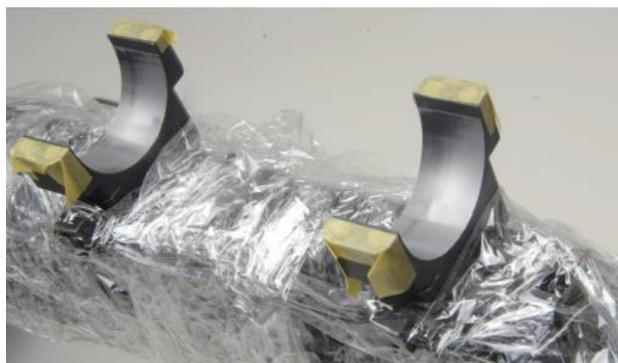
(9) Wipe off the compound carefully and install the scope with caution. Use a torque wrench to install the scope at the correct torque value.
